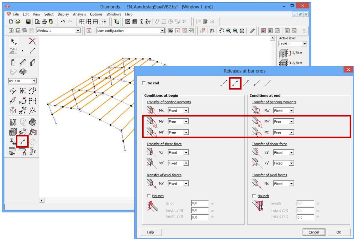
When you confirm the settings, small round symbols will appear on the ends of the girders. These indicate the presence of a hinge. In this case, we keep the torsional moment  $M_x$  fixed. If you set it free, this means the bar (girder) can rotate freely around its own axis, which is not the case.
