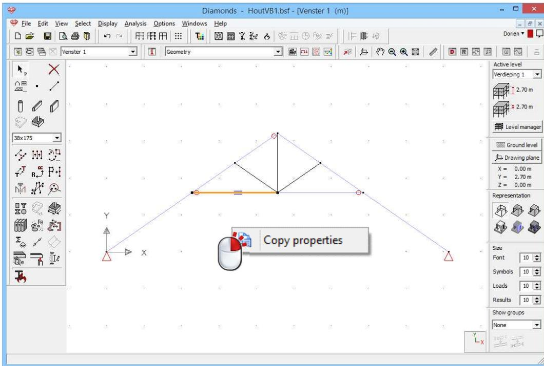
Select the option 'Copy properties'. Now select the 3 bars without cross section and material (use the SHIFT key), and click once with the right mouse button. Then paste the cross section and material on the bars.
