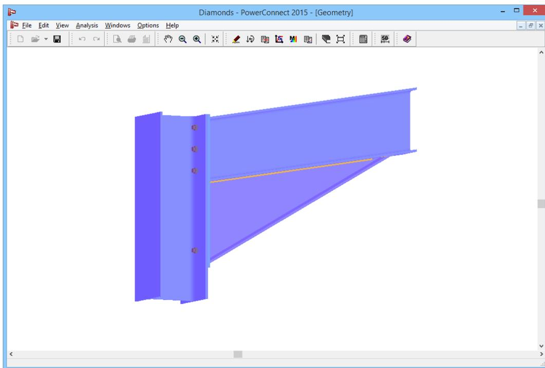
Now you can adjust the geometry of the connection. For example, select the column, then click once with the right mouse button on the column. Add a web plate.
