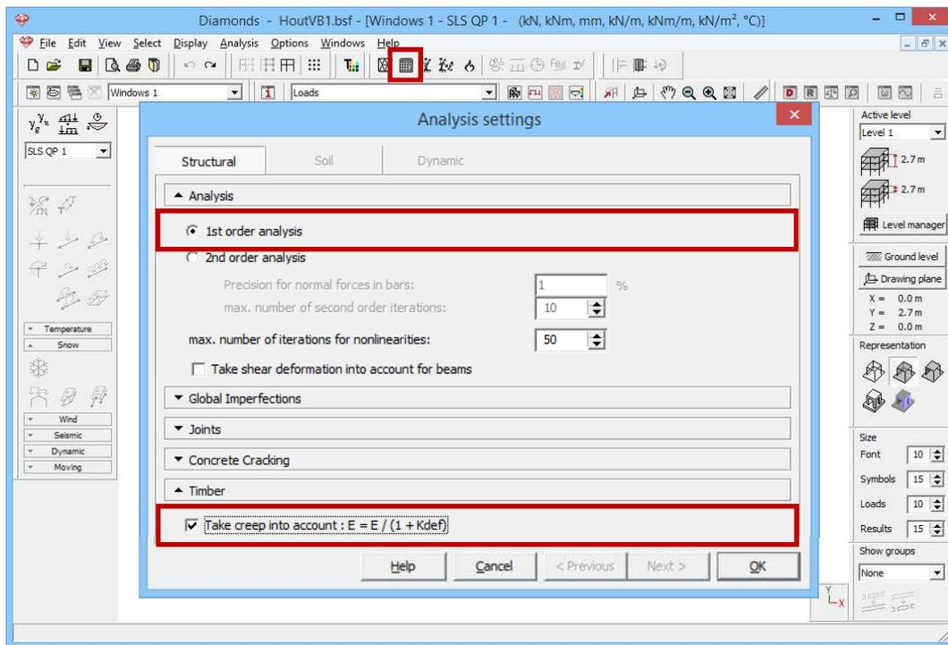
We choose a first order calculation and confirm with 'OK'. A dialog box displays the progress of the calculation.
