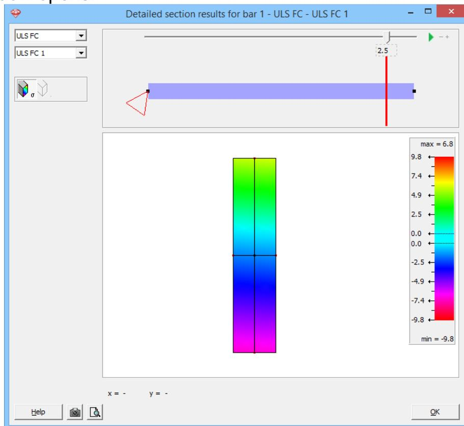
You can retrieve the results at any position using the slider. Moreover, you can also enter a distance. Consult for example the results on 2,50m. Enter '2,50' under the white arrow.
