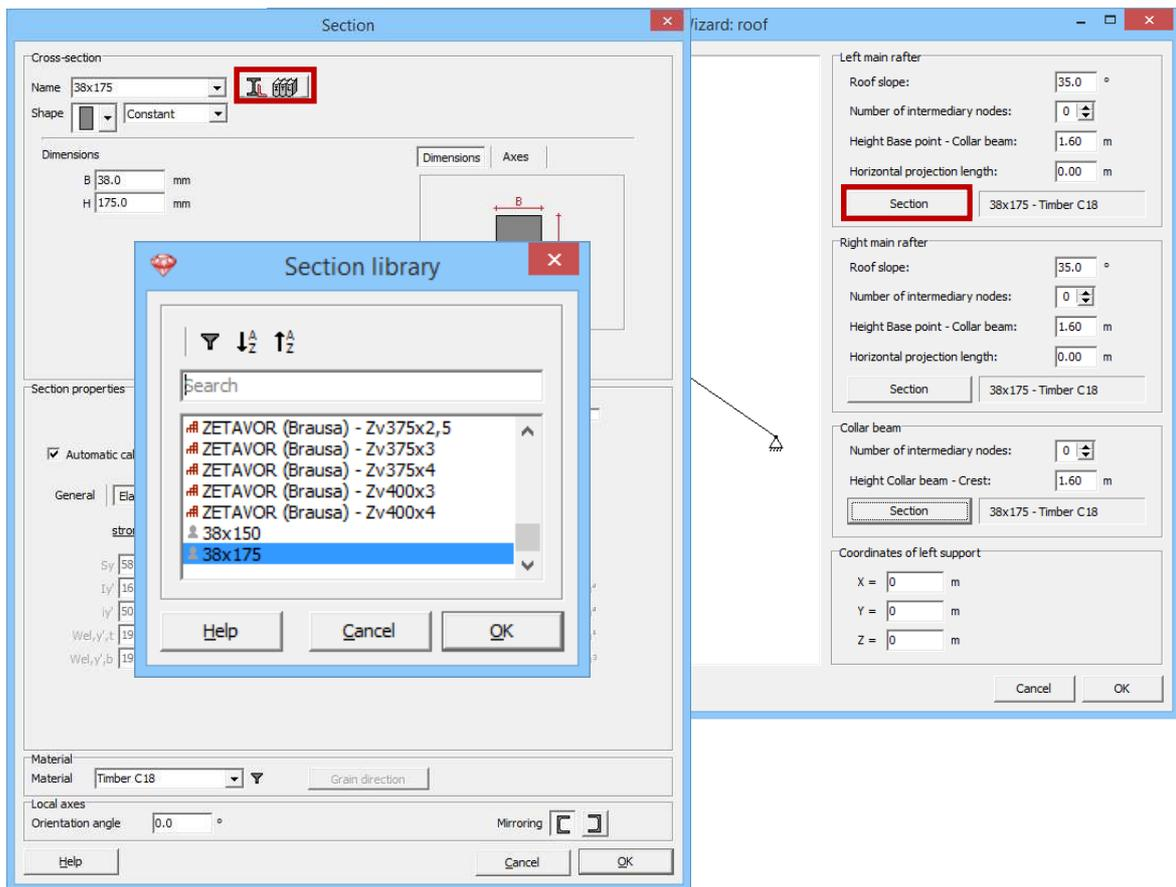
Then click on 'OK' to confirm your selection. Verify if the material is set to 'Timber C18'. Click 'OK' to assign the cross section to the beams. Then click twice 'OK' to draw the structure.
