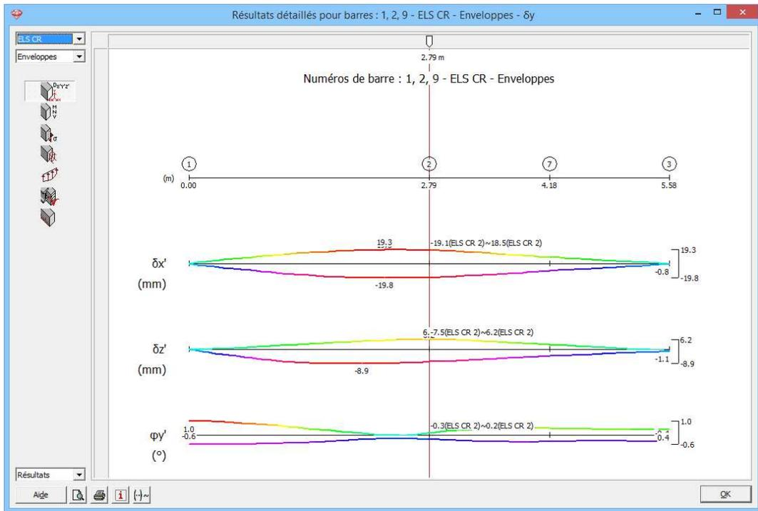
Note that in this window the deformations are defined according to the local axes of the bars. Also the angular rotations  $\varphi_{x'}$  (round the local  $x'$  axis) and  $\varphi_{y'}$  (round the local  $y'$  axis) are displayed.
