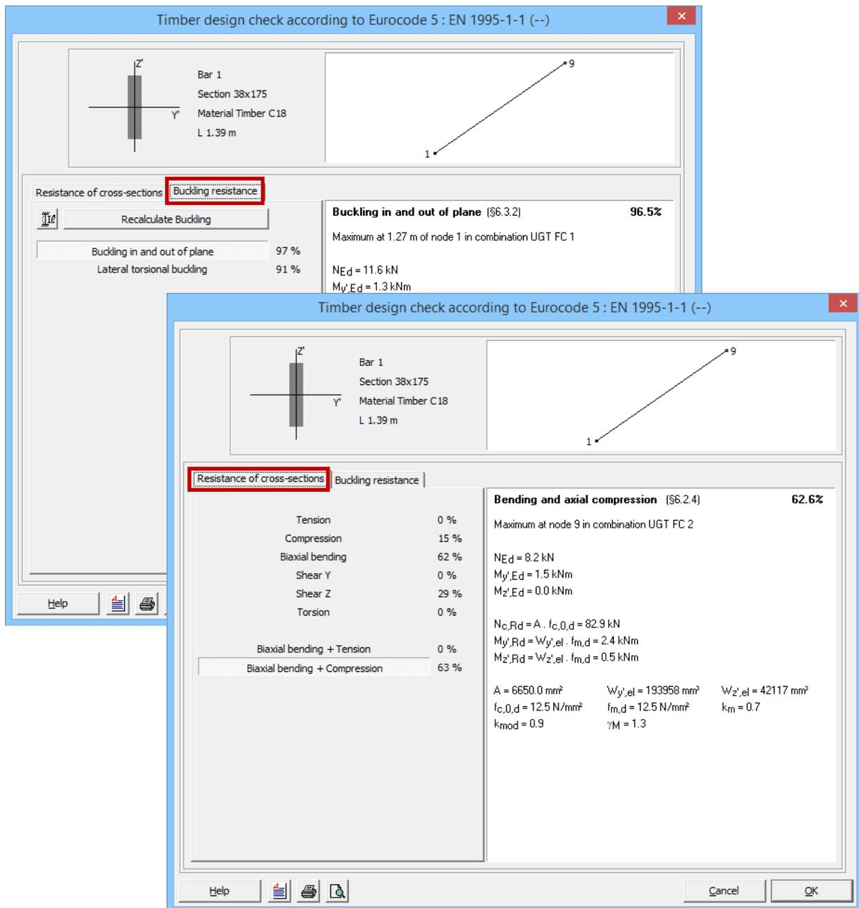
From this window we learn that both buckling and lateral torsional buckling determine the stability of the rafter. When we look at the results of the strength, the verification for bending is determining.
