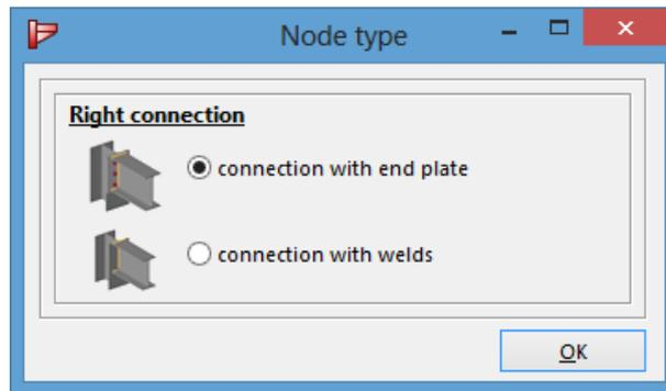
PowerConnect generates a connection based on a number default parameters.
