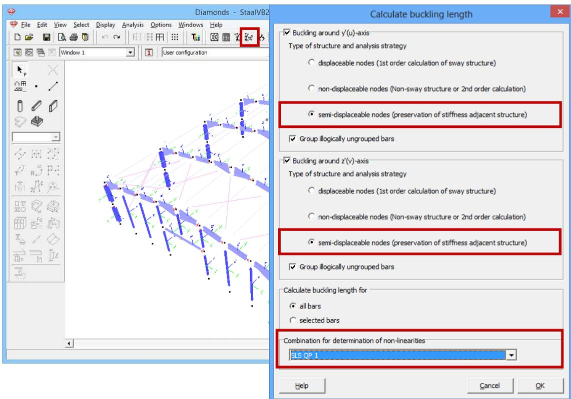
In each direction (round  $y'(u)$ - or  $z'(v)$ -axis) Diamonds asks you for which type of structure and for which type of analysis (first or second order) you would like to calculate the buckling lengths.
