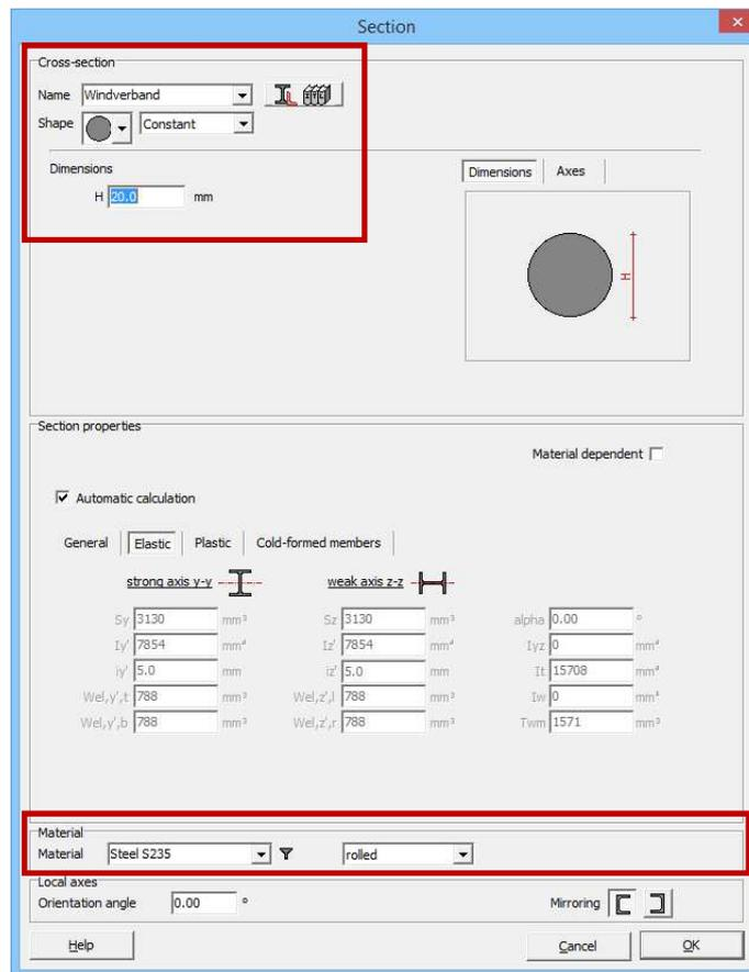
Finally, the rods must be defined as tie rods. This means that the rods can't take compression. Select the bars and click on
