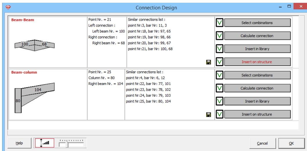
The first connection is now dimensioned. The dialog window allows you to calculate other connection, despite a new elastic analysis is actually necessary. But this way you quickly and efficiently find a solution.
