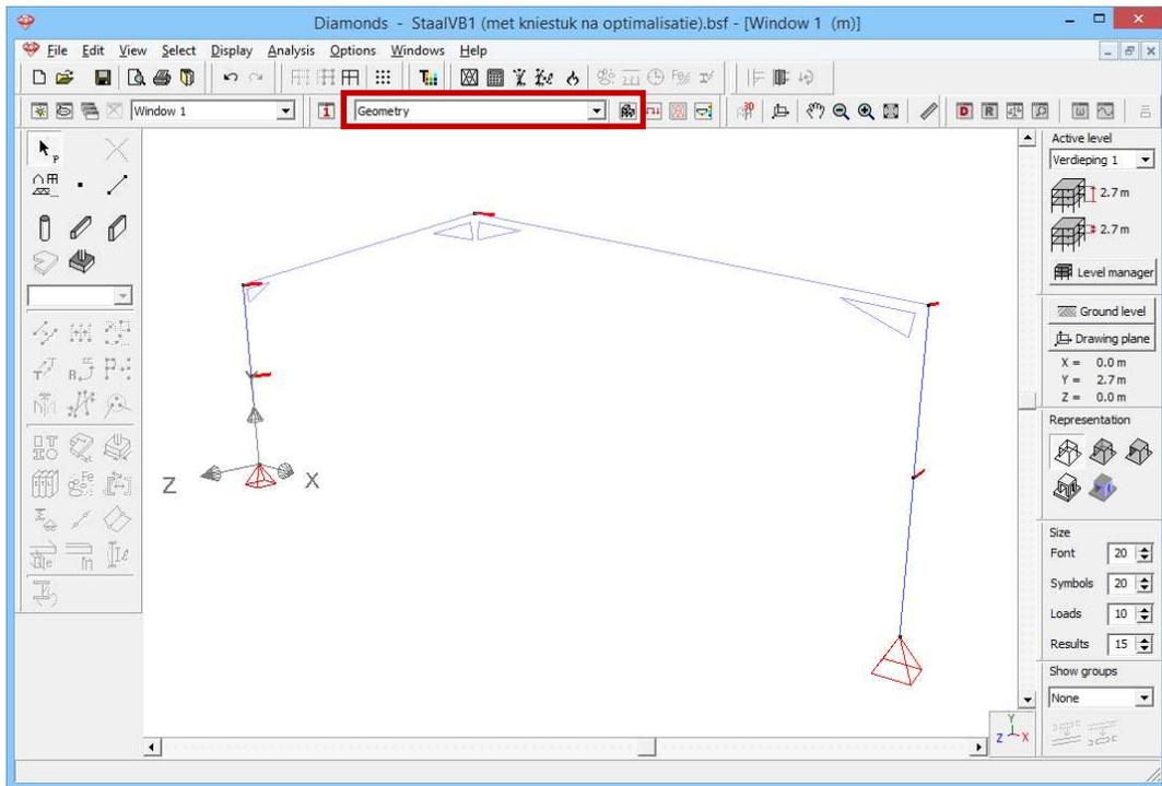
Defining the structure is always done in the 'Geometry' configuration. Click on
