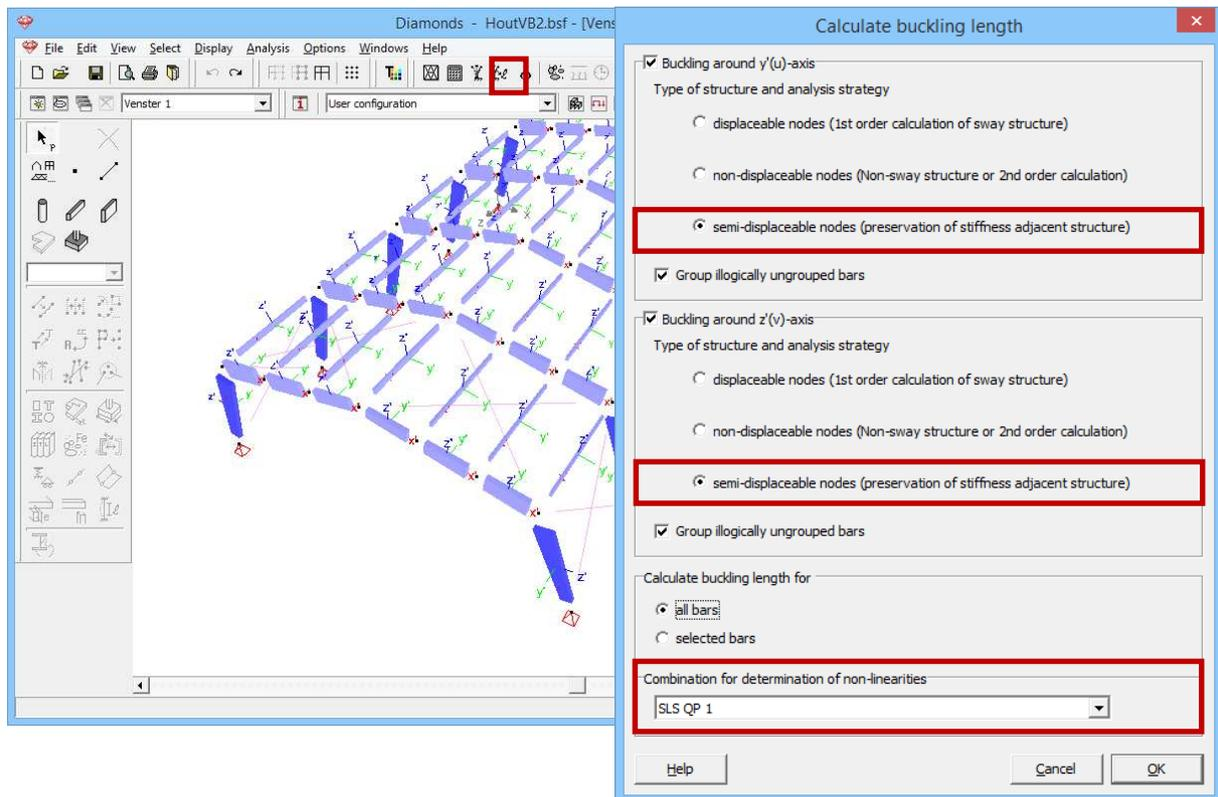
In each direction (round  $y'(u)$ - or  $z'(v)$ -axis) Diamonds asks you for which type of structure and for which type of analysis (first or second order) you would like to calculate the buckling lengths.
