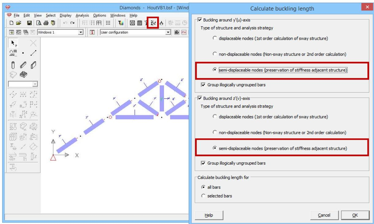
In each direction (round  $y'(u)$ - or  $z'(v)$ -axis) Diamonds asks you for which type of structure and for which type of analysis (first or second order) you would like to calculate the buckling lengths. It is important that you use the same type of analysis as what you indicate here. We choose 'semi displaceable nodes'.
