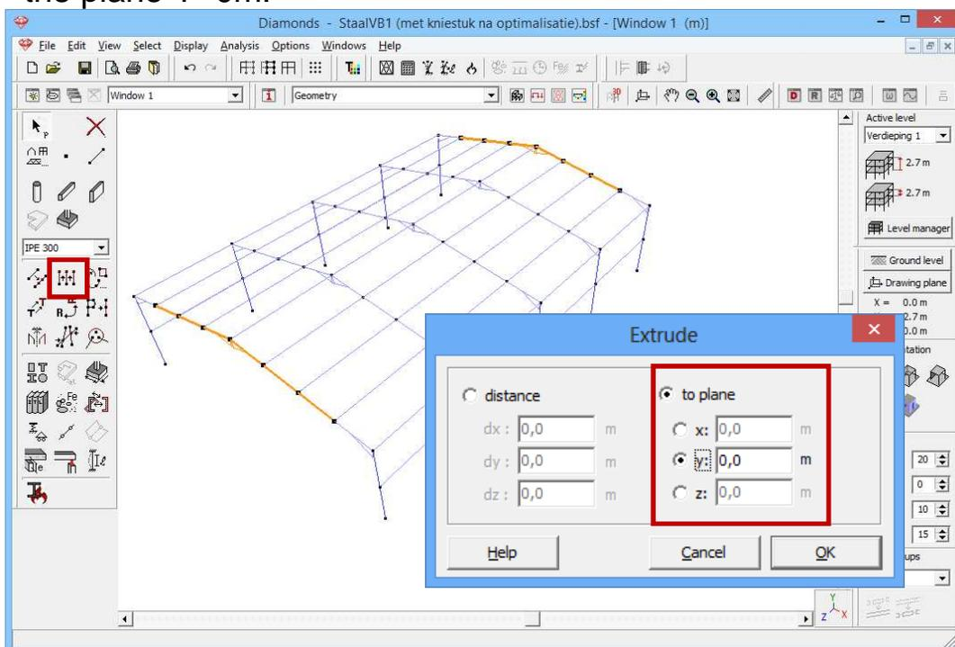
With this function we create bars with start point the selected point and end point determined by the components of the input vector.
