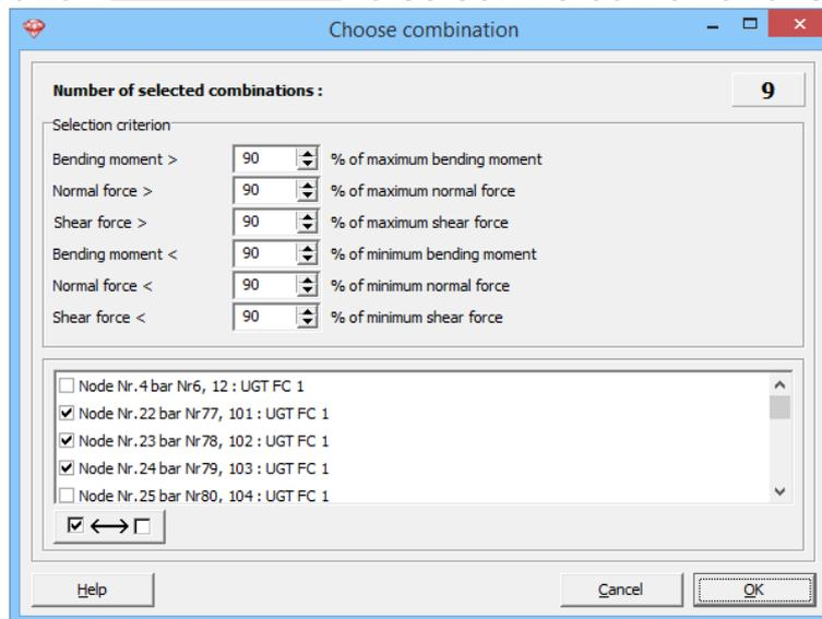
If necessary, set all percentages to 90% and click 'OK'. A 'V' will appear in front of the button **Select combinations** to indicate this step is completed for the selected connection. The combinations will be saved, even when you switch to another connection.
