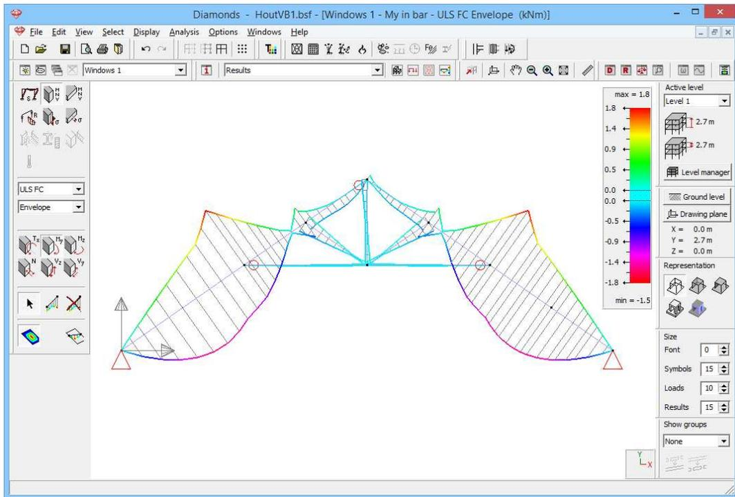
The moment diagram is always displayed on the tension side of the element. The sign of the bending moment corresponds to direction of the local axes. In this case the local  $z'$ -axis is directed upwards and causes a positive moment thus tension on the upper side.
