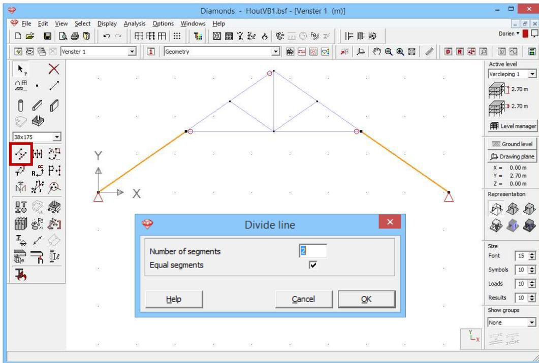
No we will prevent the movement out of the plan for all nodes, except for the two the supports.
