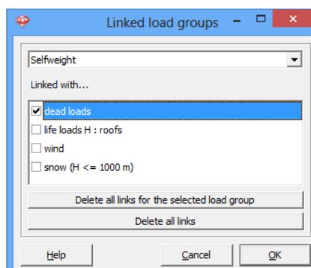
Using 'Linked load groups' will reduce the amount of load combinations and is applicable on small and large structures.
