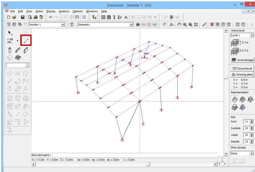
Select the just drawn line using the menu command 'Select – Section - ?' and click on
