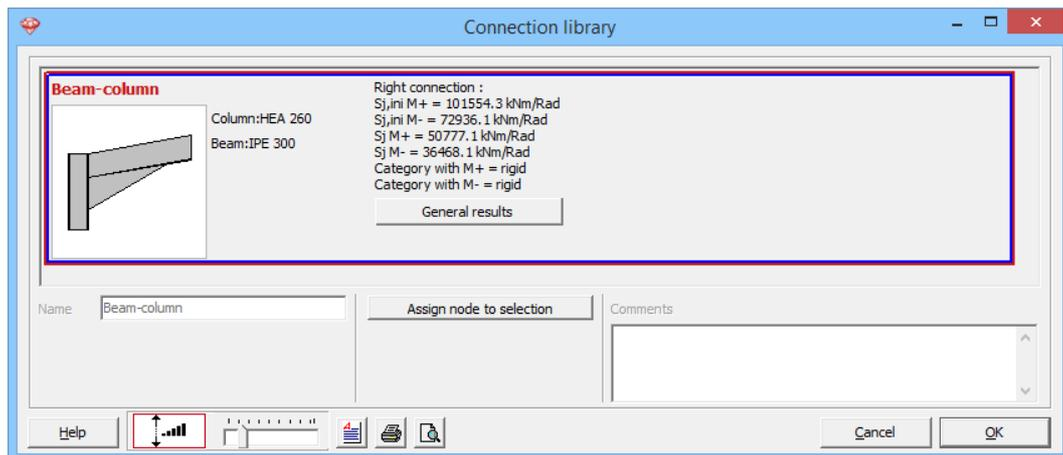
To assign the connection to the selected bars, click on [Assign node to selection](#). The name of the connection now appears in the model. The assignment of the same connection to the other nodes is done in the same manner.
