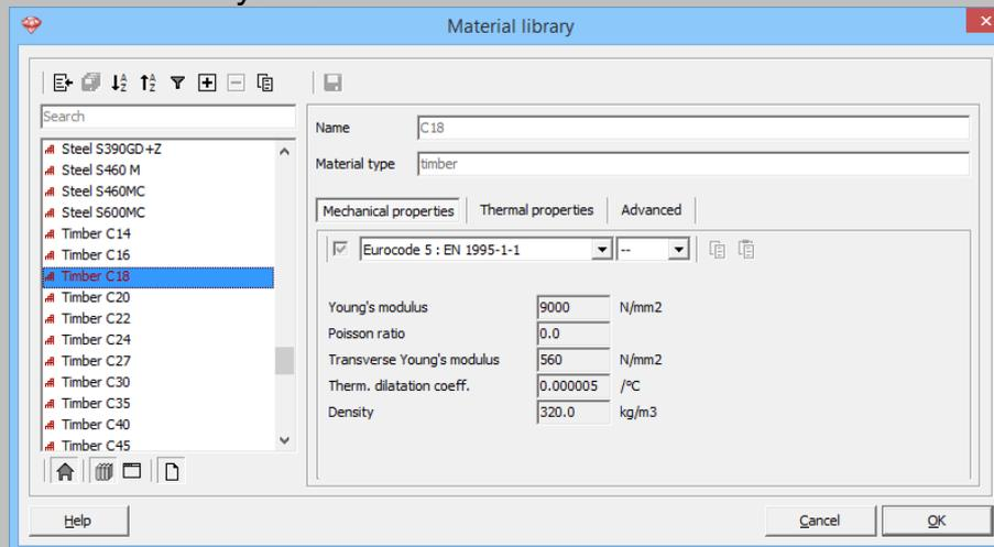
The properties of default materials are determined using the standards and can't be edited. Should you wish to make adjustments, you should make a new material. User defined materials are marked by the icon
