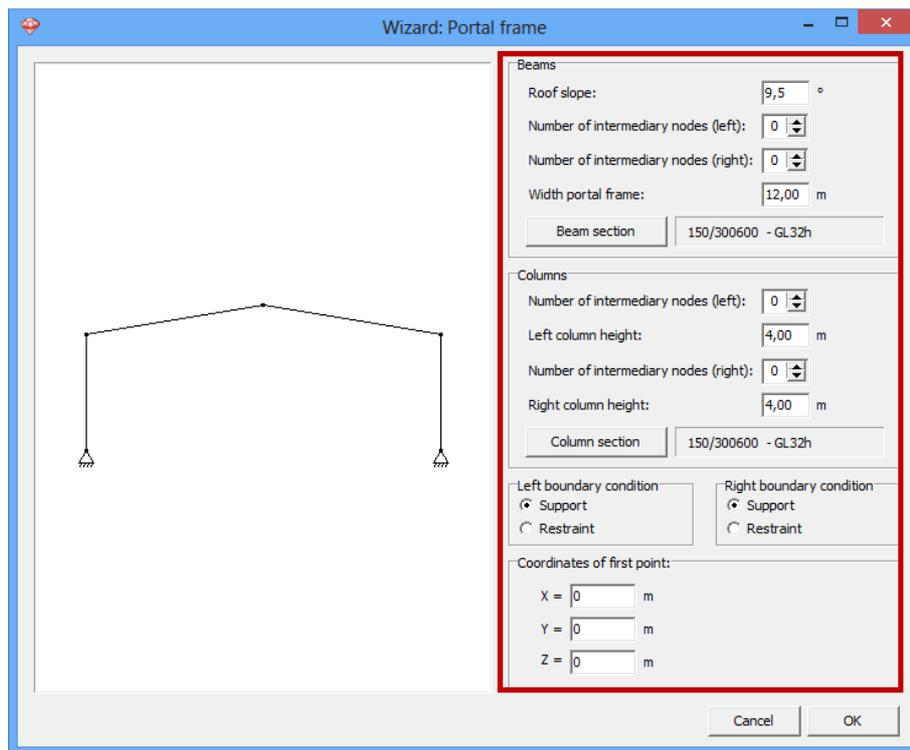
The beams and columns all have the same tapped cross-section. To change the cross section of the bars:
