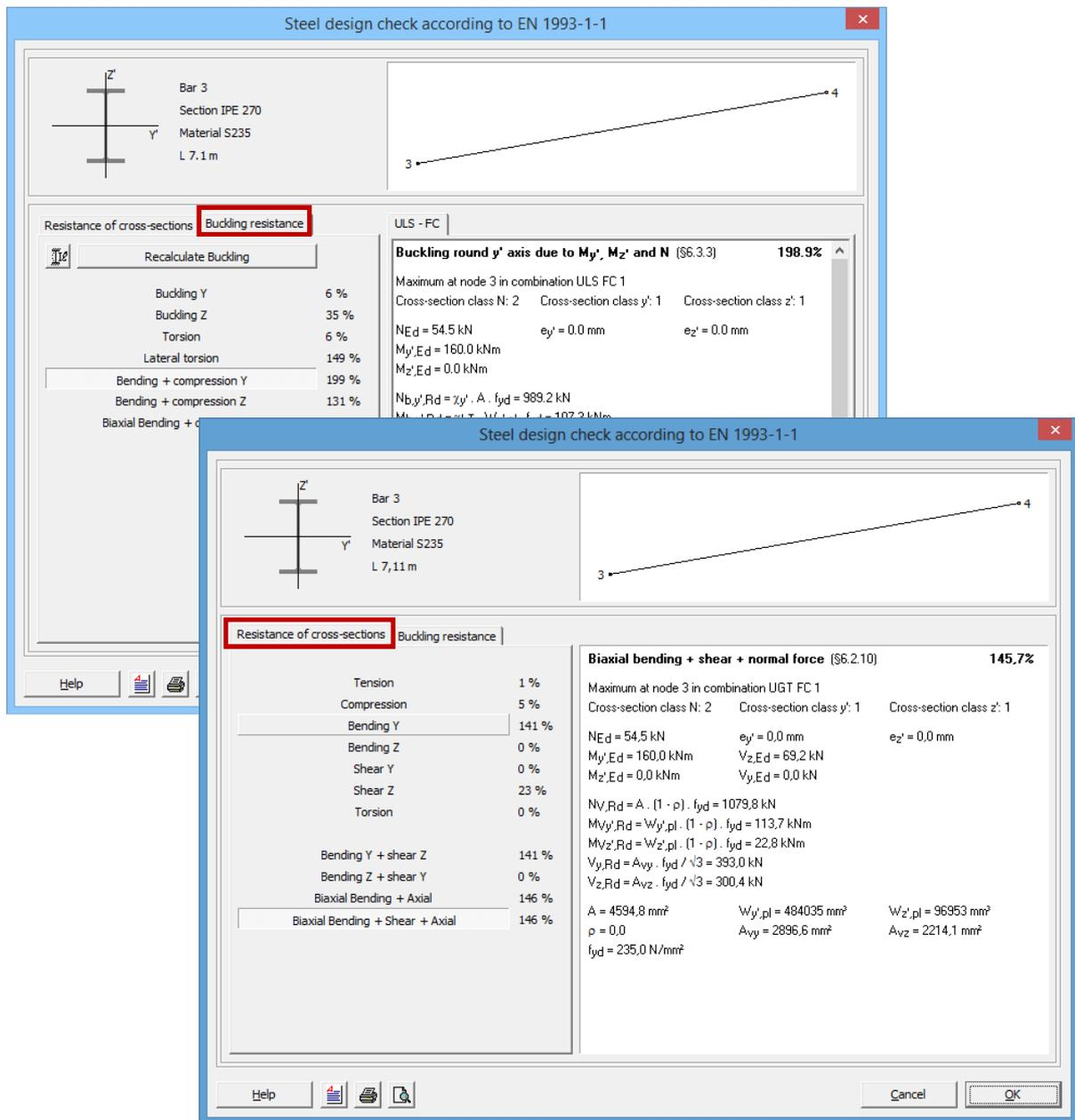
From the window about strength we learn that the check for bending + shear + axial forces gives us the highest percentage (146%). When we look at each 'check' separately, we see that bending is the determining 'check'. It gives us percentages higher than 100 AND higher than the percentages we find for axial and shear forces. The only solution is choosing a larger cross section (= larger moment of resistance) or a better material (= larger yielding stress  $f_y$ ).
