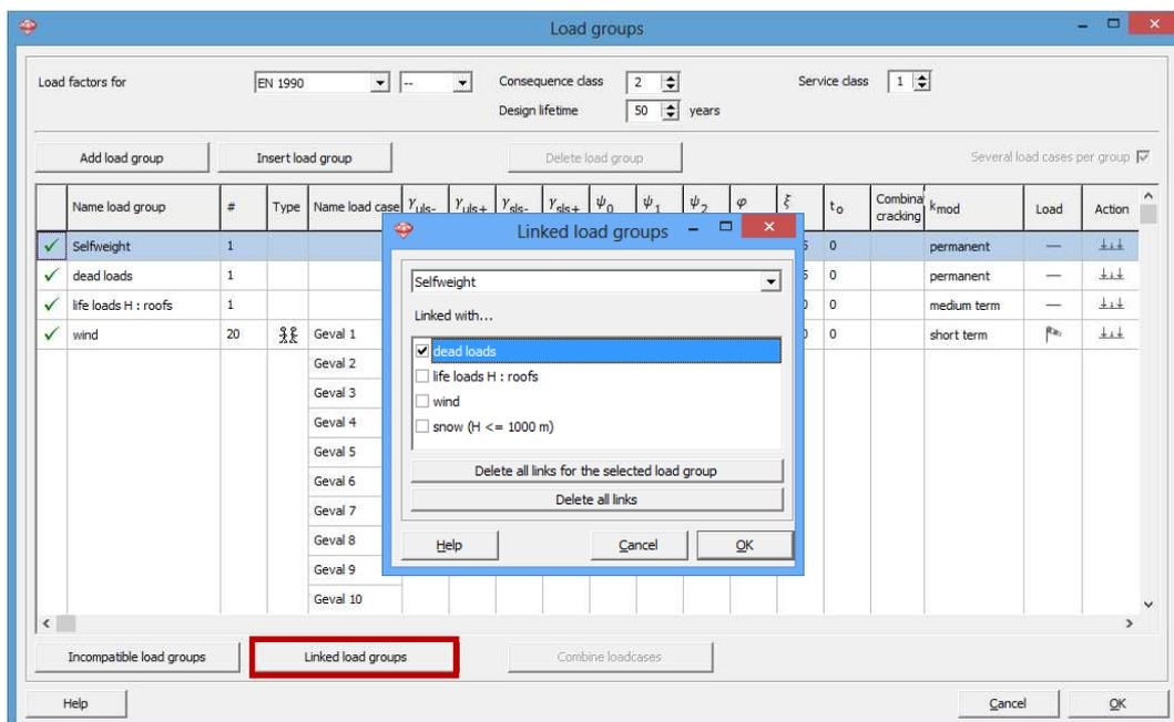
Using 'Linked load groups' will reduce the amount of load combinations and thus also the calculation time (especially noticeable on large models).
