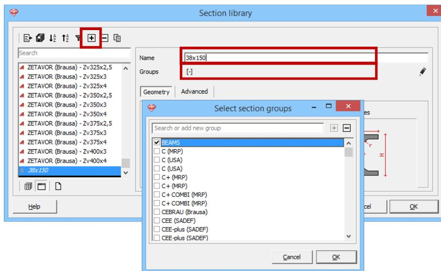
Then click on
