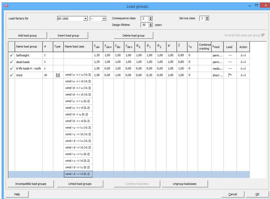
*Note: because we calculate a 2D truss, we will not generate wind out of the plane, but this can also be done with the wind generator.*
