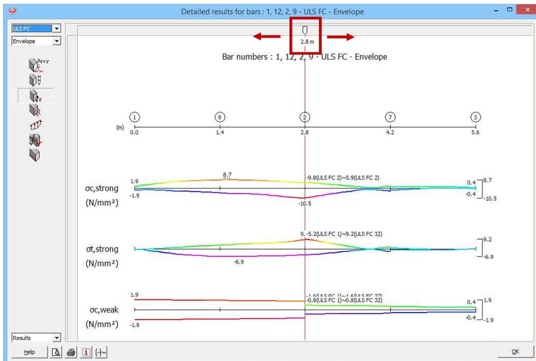
You can retrieve the results at any position using the slider. Moreover, you can also enter a distance. Consult for example the results on 2,45m. Enter '2,45' under the white arrow.
