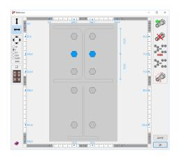
and requirements imposed by the design codes: you can either opt for a uniform distribution of bolt rows, or choose to keep distances between all rows down to the minimum. In this case, bolts will be placed as high and close together as possible.
