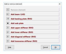
With a moment connection you could also add stiffening elements such as haunches. Again, smart references are used so that your input is minimal and you can quickly assess the effect of the stiffener.
