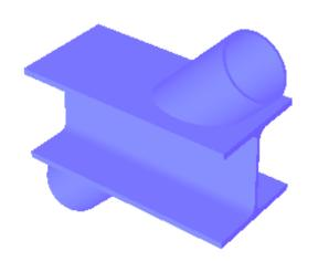
Welded tubular joints can consist of 2, 3, 4 or 5 connected elements. For the cross-sections, you have the choice between rectangular, square or round tubular profiles and I or H profiles.
