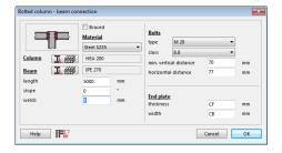
A handy wizard guides you through the definition of the various connection components. You specify the material, as well as the beam and column cross-section, bolt diameters & bolt grades, and the size of the connecting element. You also have a short-cut option here by clicking on 'OK' to leave all settings on default. For default values, PowerConnect uses smart references to the measurements of used cross-sections so that your connection turns out realistic, even with default settings.
