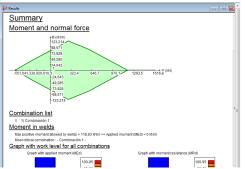
You can analyze simple column bases with I or H sections, rectangular and square tubular profiles. As anchors you have a choice between straight anchors with or without anchor plates and bent anchors. Anchors can be placed inside or outside the flanges of I profiles. With 1 click, you can add front, back, left and right stiffeners or cramp to the base plate.
